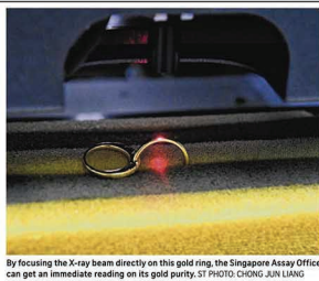
By focusing the X-ray beam directly on this gold ring, the Singapore Assay Office can get an immediate reading on its gold purity. ST PHOTO: CHONG JUN LIANG
