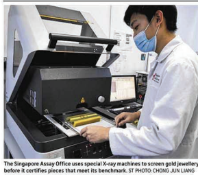
The Singapore Assay Office uses special X-ray machines to screen gold jewellery before it certifies pieces that meet its benchmark. ST PHOTO: CHONG JUN LIANG
